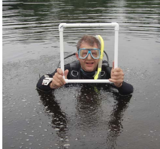
Figure 7. A quadrat is a square frame laid down on the bottom. All plant stems within the 0.1 m 2 square are counted.
