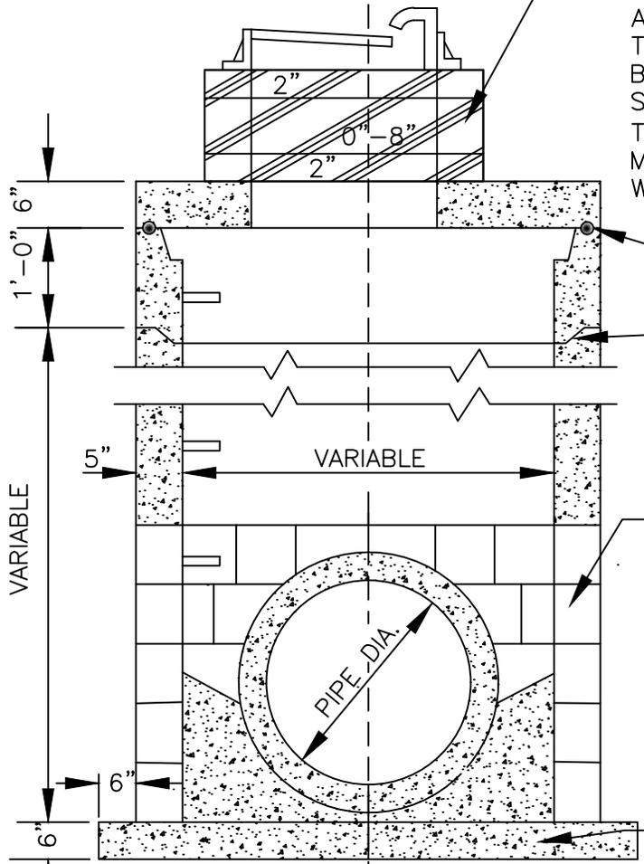
RAMNEK OR SIMILAR GASKET TYPE MATERIAL TO BE PLACED BETWEEN SLAB AND TOP OF MANHOLE SECTION.
