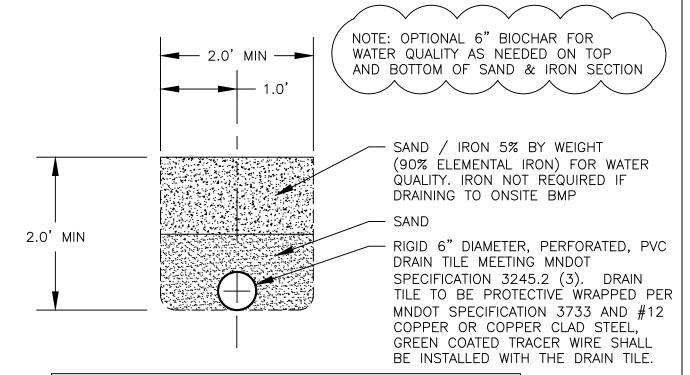
SAND USED IN EITHER SUBDRAIN EXAMPLE SHALL CONFORM TO MN/DOT SPECIFICATION 3149.2B (SELECT GRANULAR)
