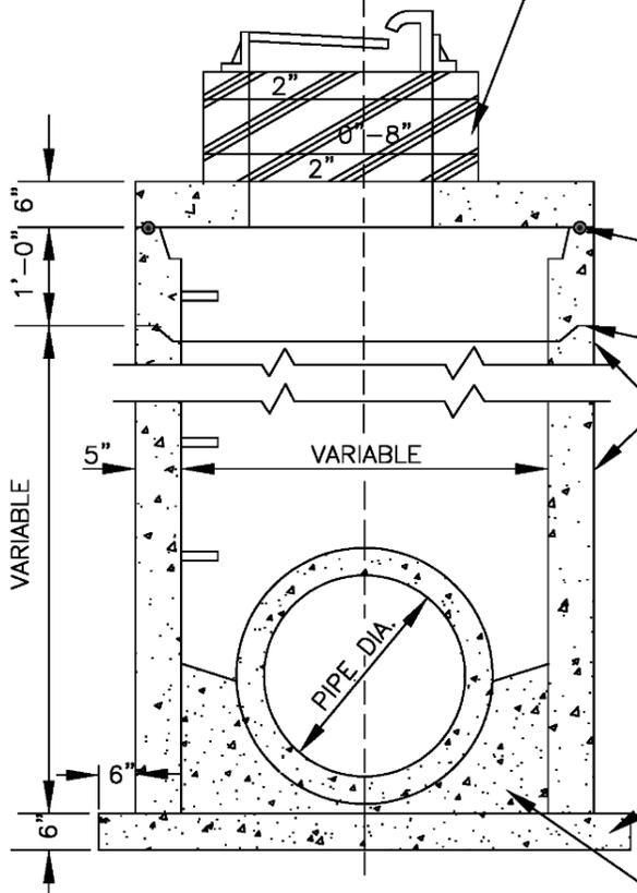
RAMNEK OR SIMILAR GASKET TYPE MATERIAL TO BE PLACED BETWEEN SLAB AND TOP OF MANHOLE SECTION.
