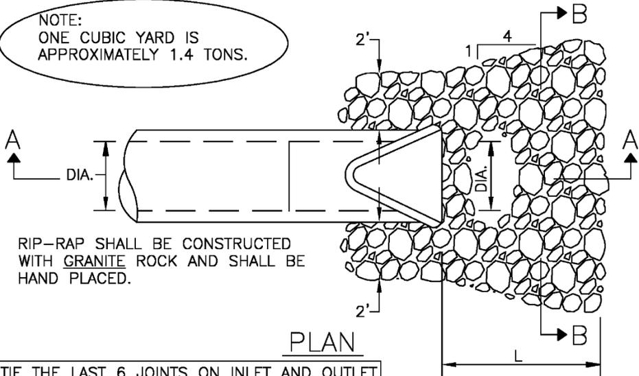
RIP-RAP SHALL BE CONSTRUCTED WITH GRANITE ROCK AND SHALL BE HAND PLACED.
