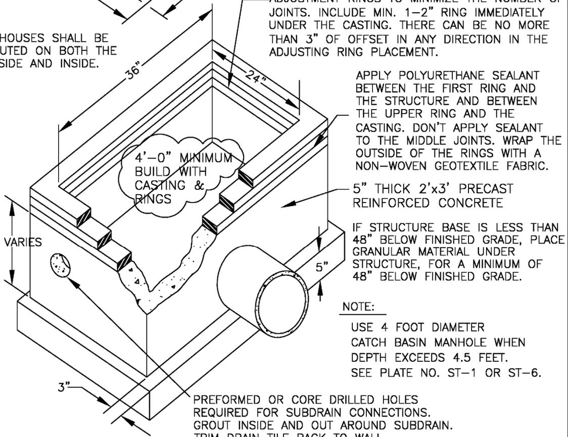
APPLY POLYURETHANE SEALANT BETWEEN THE FIRST RING AND THE STRUCTURE AND BETWEEN THE UPPER RING AND THE CASTING. DON'T APPLY SEALANT TO THE MIDDLE JOINTS. WRAP THE OUTSIDE OF THE RINGS WITH A NON-WOVEN GEOTEXTILE FABRIC.
