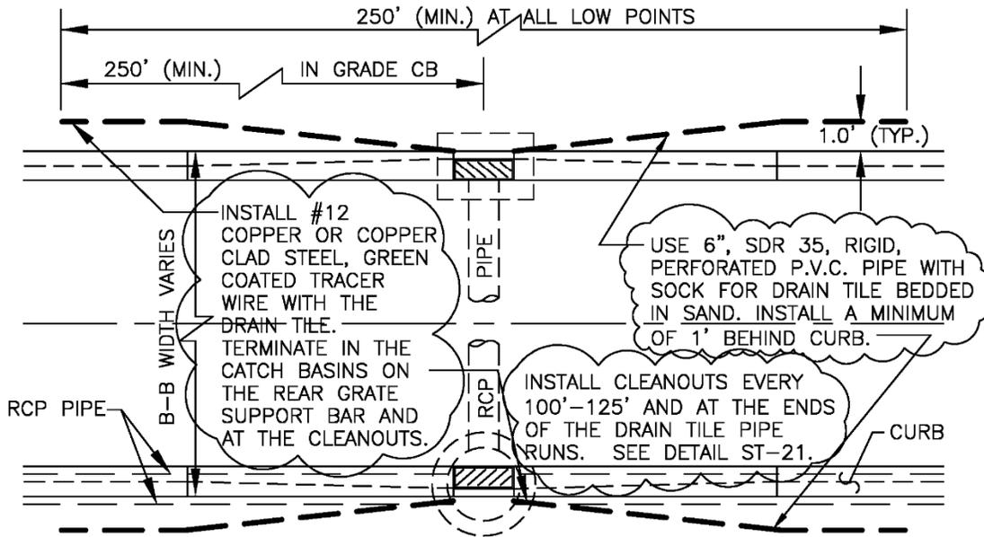
6" RIGID PERFORATED DRAINTILE IS REQUIRED AT ALL LOW POINT CATCH BASINS AND ON THE UPHILL SIDE OF ALL IN-GRADE CATCH BASINS. BENDS MAYBE USED UP TO 22 1/2 DEGREES WITH THE RIDGID DRAIN TILE. FLEXIBLE 6" DRAIN TILE CAN BE USED IN CUL-DE-SACS.
