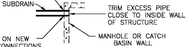
PERFORMED HOLES REQUIRED ON NEW STRUCTURES FOR SUBDRAIN CONNECTIONS. CORE DRILL SUBDRAIN HOLES FOR ANY ADDITIONAL CONNECTIONS TO NEW OR EXISTING STRUCTURES.
