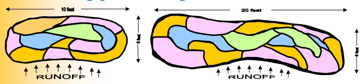
Small, 80 square foot rain garden, located less than 30 feet from the downspout will provide infiltration of a half-inch rainfall for the following areas.
