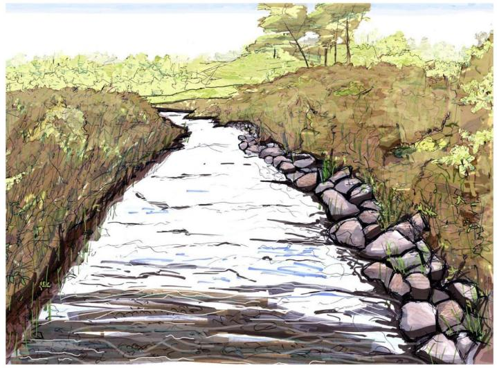
Stone Toe Protection is constructed from cobble-sized rock on the creek edges. It extends to approximately the bankfull level, which will protect the channel banks for flow events that occur every 1 to 2 years or less. The material will extend into the ground to resist scour. Coarse gravel is used to separate the larger rock material from underlying soil. Stone toe protection is typically used in conjunction with revegetation of the upper banks.
